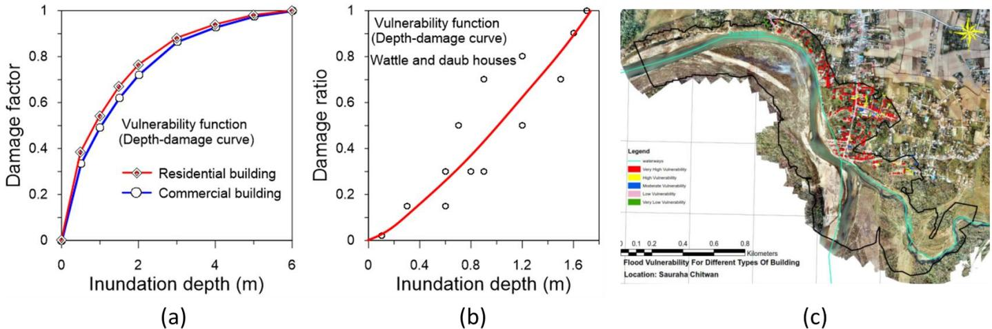
Figure: a) Depth-damage curves for residential and commercial buildings (after Huizinga et al. 2017), b) Depth-damage curve for Wattle and daub houses (after Thapa et al. (2020), and c) Flood vulnerability map with depth raster for 100 yrs flood
