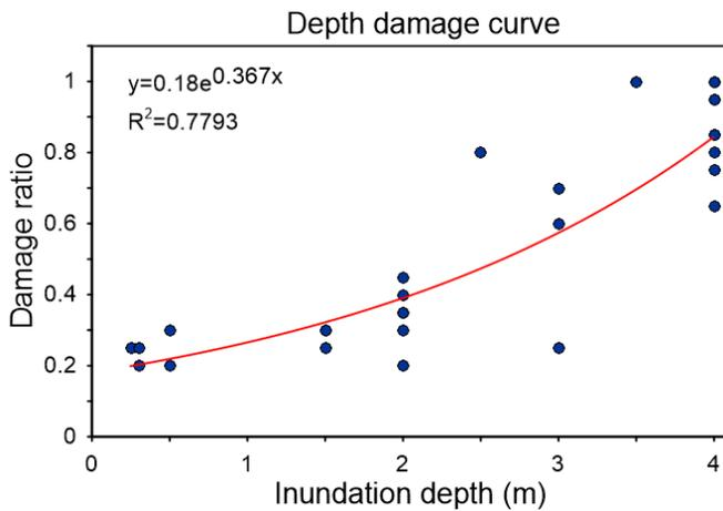
Figure 5: Depth Damage Curve – Masonry Building
