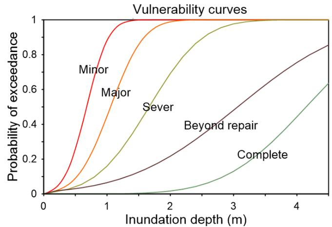
Figure 6: Vulnerability Curve for Masonry Buildings
